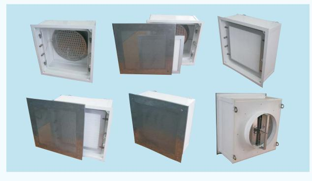
Pharmaceutical Industry has special requirement for filter system. To meet this strict standard, FLECO specially design this terminal filter with GEL sealant and unique structure.
